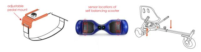
Slide on all the protective rubber pedal mount covers on each end of the pedal mounts. Then using the hook and loop straps, place the hook and loop side of strap downward and then pull each strap end through the holes on back of each pedal mount.
