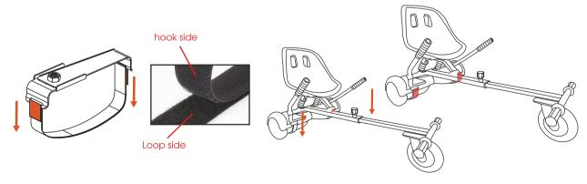
**WARNING:** Do not overtighten straps when you are assembling your HK5 KART to your scooter. Ensure that the HK5 KART is secure to the scooter when attaching. Ensure the foam pads are attached to the bottom of the pedal mounts so that the HK5 KART does not touch the footpad sensors on the scooter. See below diagram for correct fitting. The foam pads are to give extra pressure support to the pedal mounts.
